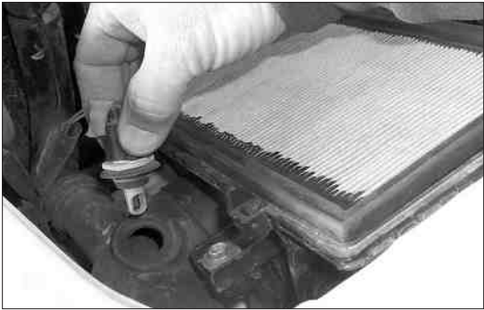
11. Remove the air temp sensor by pulling in an upward direction as shown.
