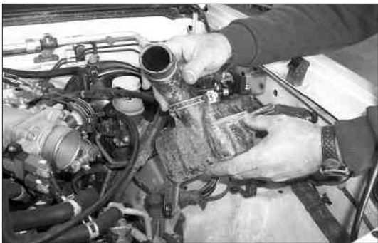
20. Remove the resonator box as shown.
