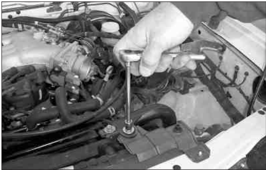
16. Remove bolt from front of resonator using a 10mm socket. NOTE: Bolt will be re-used.
