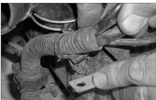
19. Using pliers, remove the wire loom clip.
