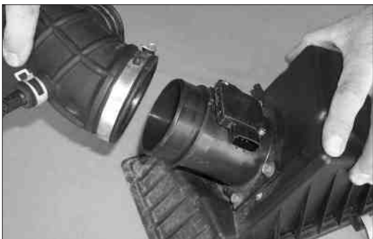
21 Loosen hose clamp using an 10mm socket and remove air duct tube from mass air sensor.
