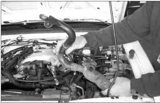
17. Remove the front resonator assembly as shown.
