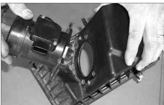
22. Remove the four bolts from mass air sensor housing using a 10mm socket and detach from airbox.
