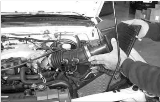
10. Unlatch the four clips on the air filter housing and remove the top assembly.
