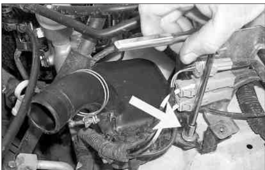
18. Remove the two bolts on rear resonator box using a 10mm socket.
