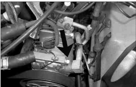
29. Remove the AC compressor mounting bolt.
