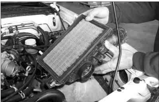
14. Remove the lower air filter housing as shown. NOTE: K&N Engineering, Inc., recommends that customers do not discard factory air intake.
