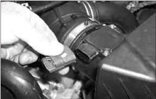
2. Disconnect the mass air sensor electrical connection.
