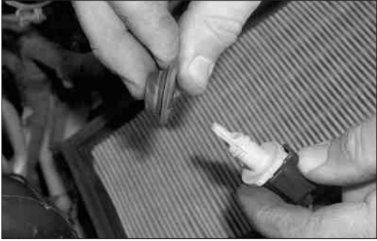
12. Remove rubber grommet from air temp sensor then disconnect the electrical connection and remove temp sensor from vehicle.
