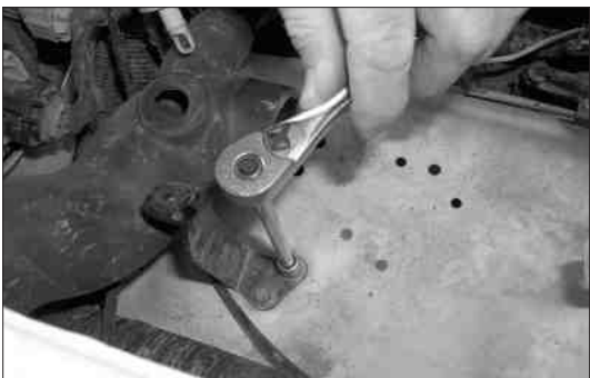
15. Remove the front support bracket using a 10mm socket.
