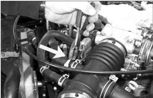
4. Squeeze the two hose clamps and slide back using pliers.
