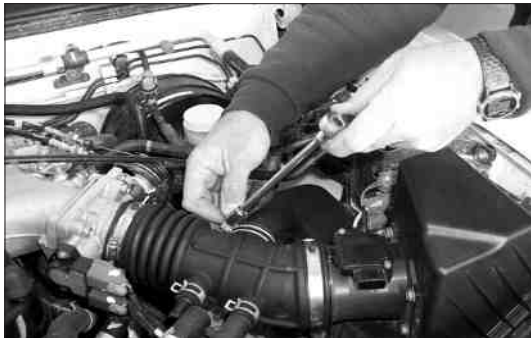
7. Loosen clamp on the resonator tube using a 10mm socket.
