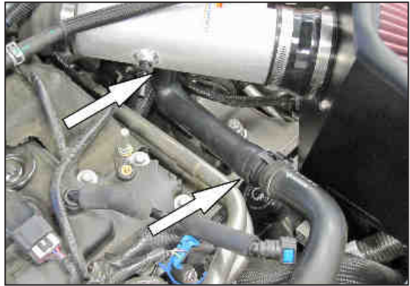
27. On vehicles equipped with air injection, install the air injection hose onto the K&N® intake tube and then connect it with the factory air injection tube.
