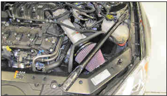
30. Reinstall the body brace and secure with the factory hardware.
