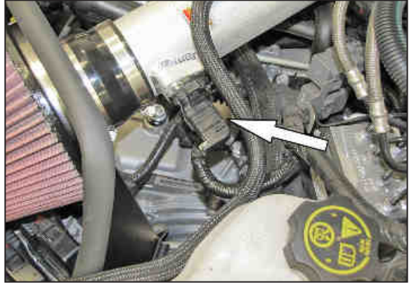
29. Reconnect the Mass air sensor electrical connection.
