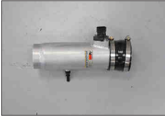
22. Install the provided hose (08496) onto the intake tube as far as it will slide on, do not tighten at this time.
