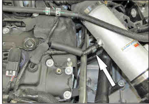
28. Connect the factory crank case vent hose to the fitting installed into the K&N® intake tube as show.
