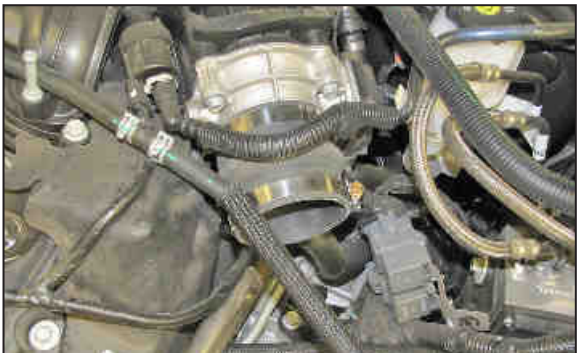
18. Install the provided hump hose (08696) onto the throttle body and secure with the provided hose clamp.
