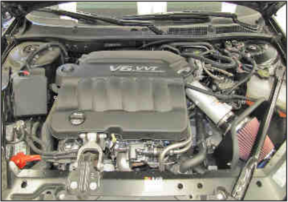
32. Reconnect the vehicle's negative battery cable. Double check to make sure everything is tight and properly positioned before starting the vehicle.
