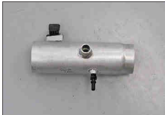
13. Install the provided NPT quick disconnect fitting into the K&N® intake tube as shown. NOTE: Plastic NPT fittings are easy to cross thread. Install the vent fitting “hand” tight, then turn it two complete turns with a wrench.
