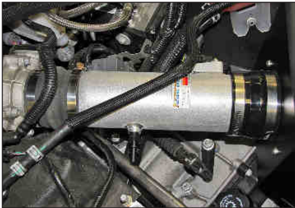
23. Install the K&N® intake tube into the hose at the throttle body and align the tube with the filter adapter. Slide the hose into position and secure with the provided hose clamps.
