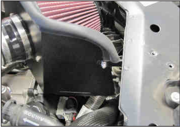
24. Secure the heat shield to the mounting bracket with the hardware provided.
