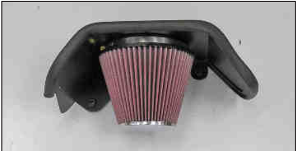
17. Install the air filter onto the filter adapter and secure with the provided hose clamp. NOTE: Drycharger® air filter wrap; part # RF-1048DK is available to purchase separately. To learn more about Drycharger® filter wraps or look up color availability please visit http://www.knfilters.com ®.
