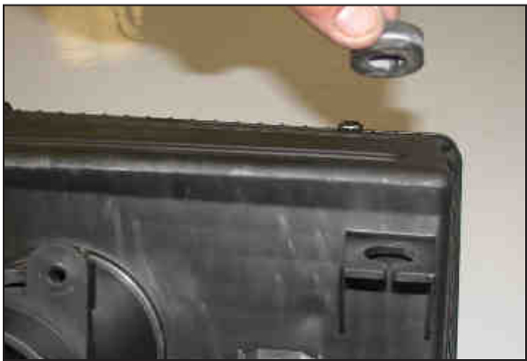
18. Remove the stock grommets from the air cleaner assembly as shown.
