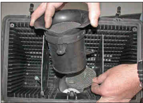
22. Remove the stock screen from the air cleaner cover as shown.
