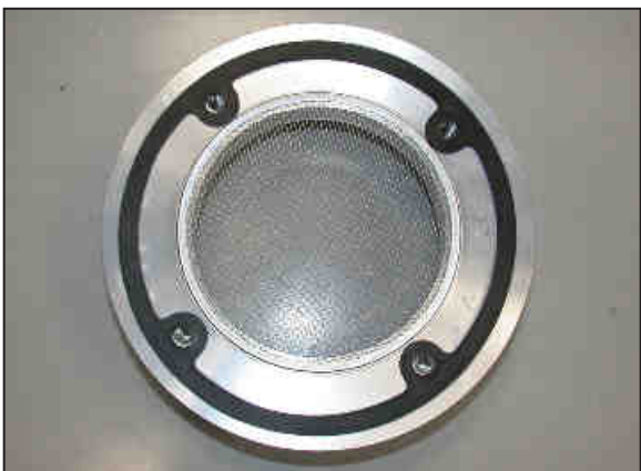
23. Install the stock screen and the provided gasket onto the back of the provided filter adapter as shown.
