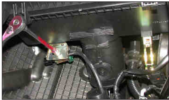
13. On manual transmission vehicles (automatic transmission vehicles go to step 14) turn the air cleaner upside down to remove the nut that secures the vacuum switch to the air cleaner assembly then remove the vacuum switch.
