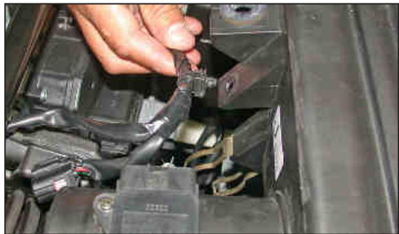
12. Using a pair of pliers, unclip the wire harness from the air cleaner assembly as shown.
