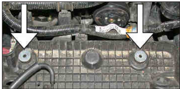
28. Install the provided rubber washers and fender washers onto the existing air cleaner mounts as shown.
