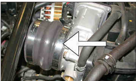
27. Install the silicone hose and hose clamps onto the throttle body as shown.
