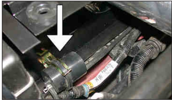
31. Manual trans only, slide the canister from step 5 into the canister clip as shown.
