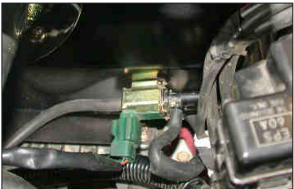
38. Reconnect the vacuum switching valve electrical connection as shown.
