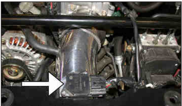
37. Reconnect the mass air sensor electrical connection as shown.
