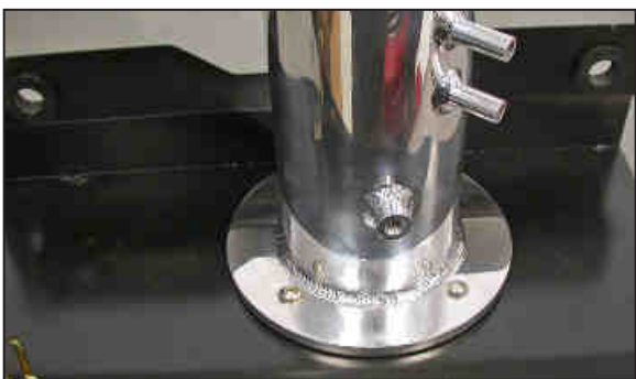
25. Install the K&N® intake tube onto the heat shield and secure with the provided hardware as shown.
