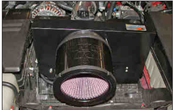
36. Install the K&N® air filter and secure using the provided hose clamp as shown.
