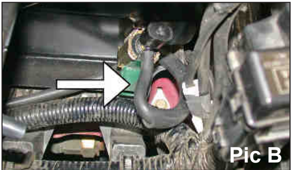
34. Manual transmission vehicles reroute the vacuum hose through the corner of the heat shield (Pic A) and reconnect the hose to the vacuum switching valve (Pic B) as shown.
