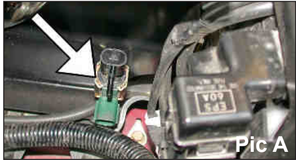
31. Manual trans only, slide the canister from step 5 into the canister clip as shown.
