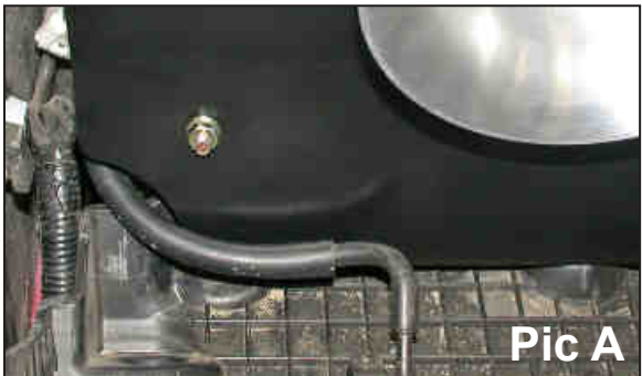
33. EU and UK SP-vehicles with the dummy electrical connection described in step 4, secure the excess electrical connector away using the zip tie provided as shown.
