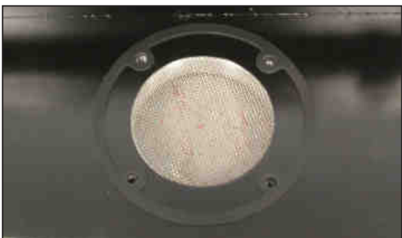
24. Install the heat shield and the remaining gasket onto the filter adaptor as shown.
