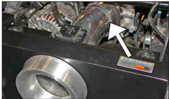
29. Install the heat shield into the vehicle and slide the intake tube into the silicone hose as shown.
