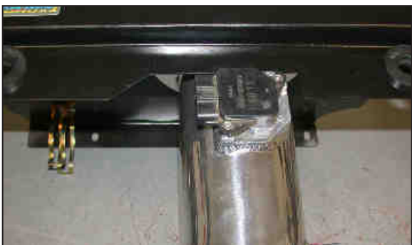
26. Install the mass air sensor into the intake tube using the provided hardware as shown.
