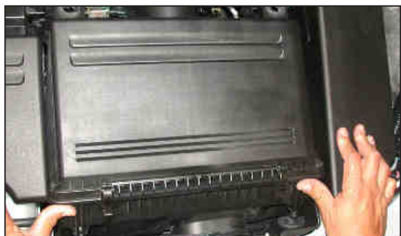
10. Push back on the front of the air cleaner to release the air cleaner from the stock grommets.
