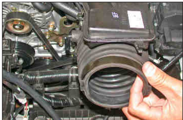
15. Remove the intake hose as shown.
