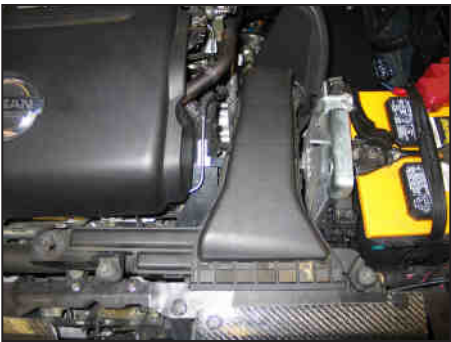
21. Reinstall the intake duct onto the core support and into the heat shield assembly. Secure with the factory bolts.
