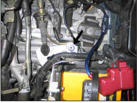
19. Install the longer rubber mounted stud onto the front airbox mounting bracket as shown. NOTE: Be sure to place a large fender washer on each side of the mounting bracket.
