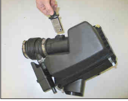
23. Remove the two screws securing the mass air sensor, then remove the mass air sensor from the stock airbox as shown.
