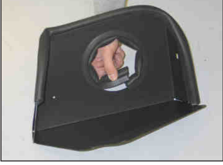
15. Install the provided edge trim into the hole of the heat shield as shown. NOTE: Some trimming of the edge trim will be necessary.
