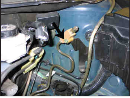
13. Remove the slave cylinder bleeder bolt shown. NOTE: Vehicles equipped with an automatic transmission will not have a bolt in this location.
