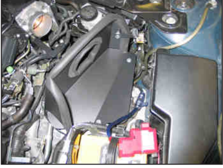
20. Install the heat shield assembly onto the rubber mounted studs installed in the previous steps and secure with the provided hardware. Secure the heat shield mounting bracket to the slave cylinder bleeder using the factory bolt. On automatic equipped vehicles, secure the heat shield mounting bracket to the bracket on the strut tower with the provided hardware.
