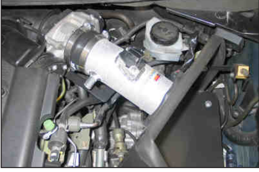
26. Install the K&N® intake tube into the silicone hose installed onto the throttle body and then align it with the tube mounting bracket. Secure the intake tube with the hardware and hose clamp provided.
