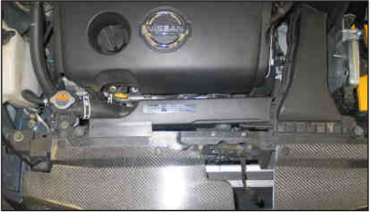
22. Reinstall the fresh air intake scoop and secure with the factory bolt.
