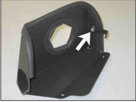
17. On manual transmission equipped vehicles, install heat shield mounting bracket #07195 onto the heat shield as shown. On automatic transmission equipped vehicles, install heat shield mounting bracket #010040.
