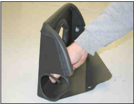
16. Install the provided quarter edge trim into the hole of the heat shield as shown. NOTE: Some trimming of the edge trim will be necessary.
