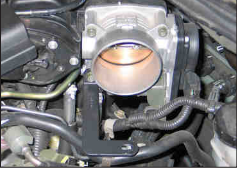
12. Using the bolt removed from the previous step, install the provided tube mounting bracket (070113) onto the throttle body as shown.
