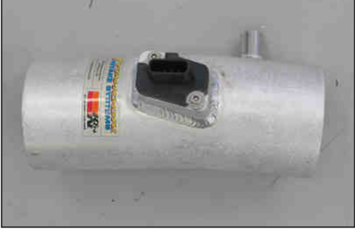
24. Install the mass air sensor into the K&N® intake tube and secure with the provided hardware.
