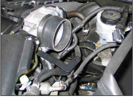
25. Install the silicone hose (084031) onto the throttle body and secure with the provided hose clamp.
