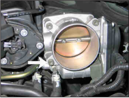
11. Remove the lower front throttle body mounting bolt shown. This bolt will be reused in the next step.
