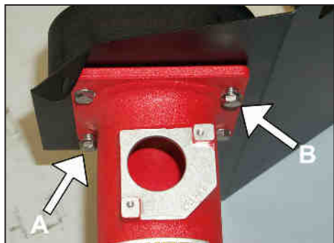
14. Assemble the intake tube, gaskets, heat shield, and filter adapter using the provided hardware as shown. NOTE: Install the lower bolt, (arrow A) and the upper bolt, (arrow B) loose as shown.
