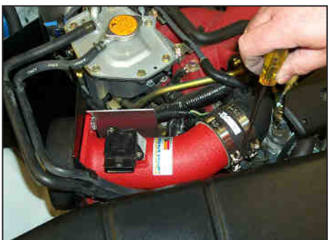
27. Tighten the hose clamp at the silicone hose as shown.
