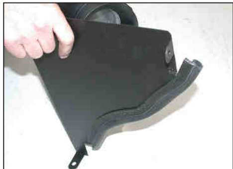
16. Install the provided edge trim onto the heat shield and trim as shown. NOTE: Some trimming of the edge trim may be necessary.
