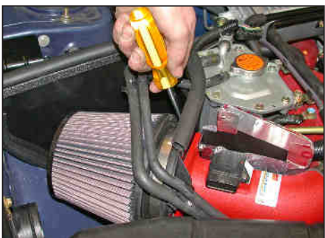
29. Install the K&N® air filter and and secure with the provided hose clamp as shown.
