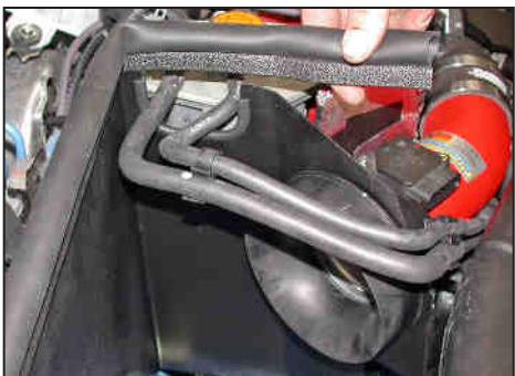
28. Install the remaining trim seal onto the heat shield and trim to fit as shown. NOTE: Some trimming of the edge trim may be necessary.
