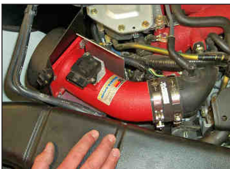
21. Install the complete assembly into the vehicle and slide the tube into the silicone hose as shown.
