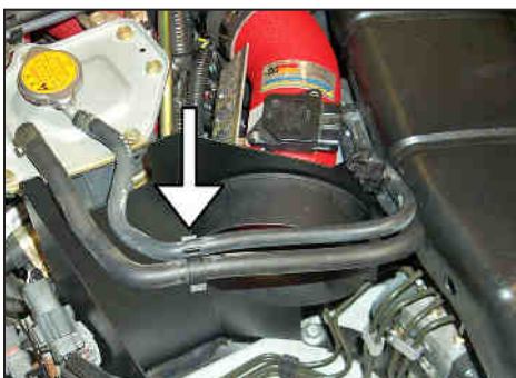
23. Reinstall the hose clip from step 22 and locate as shown.
