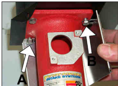
15. Install the heat insulation plate on the intake tube flange and secure it to the bolts "A" and "B" as shown.
