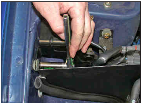
25. Using the bolt removed in step 10, secure the heat shield to the inner fender bracket but do not tighten at this time.
