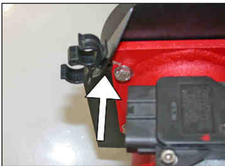
20. Install the hose clip from step 19 onto the heat shield as shown.
