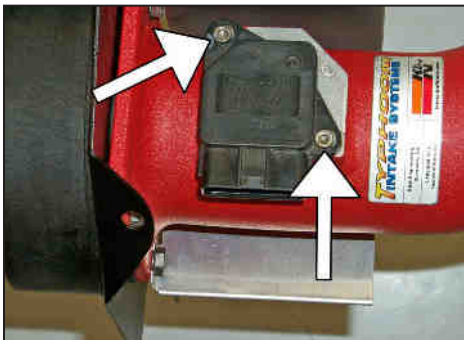
18. Install the mass air sensor from step 7 into the K&N® intake tube and secure with the provided hardware as shown.
