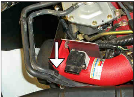
24. Secure the coolant hoses to the hose clip on the heatshield as shown.
