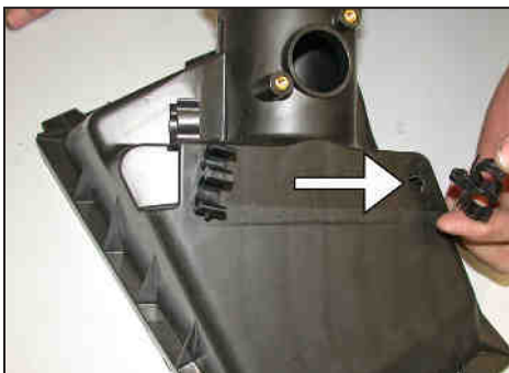
19. Remove one of the hose clips from the stock airbox assembly as shown.
