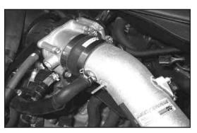
25. Connect the crank case vent hose to the fitting on the K&N $^{\otimes}$  intake tube; secure with the factory spring clamp.
