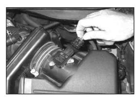
2. Disconnect the mass sensor electrical connection by depressing the center tab and gently pulling the harness away from the mass air sensor. Release the two wiring harness clips from the air box lid.
