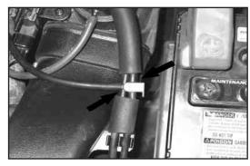
8. Disconnect the two vacuum lines from the factory "T" fitting.
