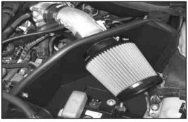
32. Install the K&N<sup>®</sup> air filter onto the K&N<sup>®</sup> intake tube; secure with the provided hose clamp.
