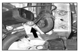
14. Install the rubber mounted stud onto the air box mounting bracket in the forward mounting hole location as shown in the photograph.
