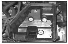
12. Remove the air filter. Remove the three bolts that secure the lower air box to the mounting bracket.
