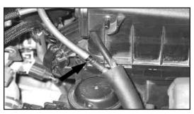
6. Disconnect the intake tube plenum vacuum line.
