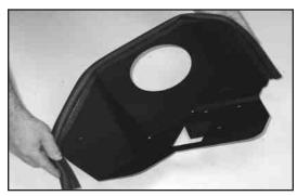
15. Install the edge trim onto the heat shield. Note: Some trimming of the edge trim may be necessary.
