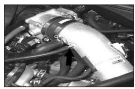
30. Install the supplied vacuum hose to the K&N® Intake Tube.
