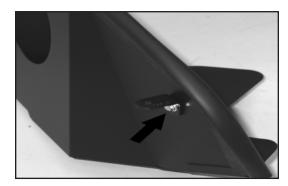
16. Install the "L" bracket (070066) onto the heat shield.
