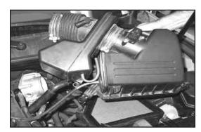
11. Release the clamps that secure the upper air box. Remove the upper air box and intake tube assembly.
