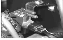
26. Install the two vacuum cap plugs onto the "vacuum switching valve."
