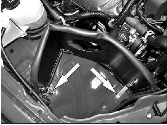
14. Install the heat shield into the vehicle using the hardware provided and the factory air box retaining nut. NOTE: The front heat shield bracket will be secured to the front air box retaining bolt location.
