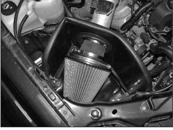
24. Install the air filter assembly onto the K&N® intake tube and secure with the provided hose clamp.
