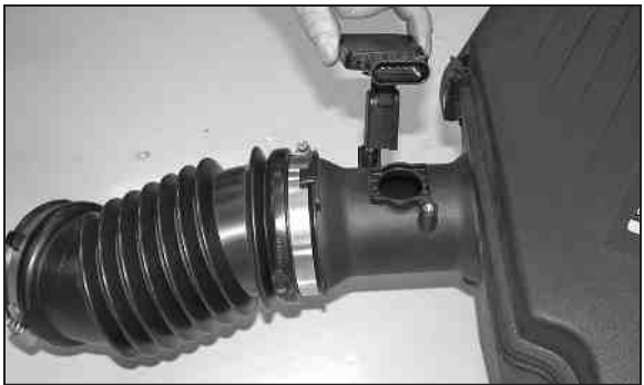
15. Remove the mass air sensor from the stock air box as shown.
