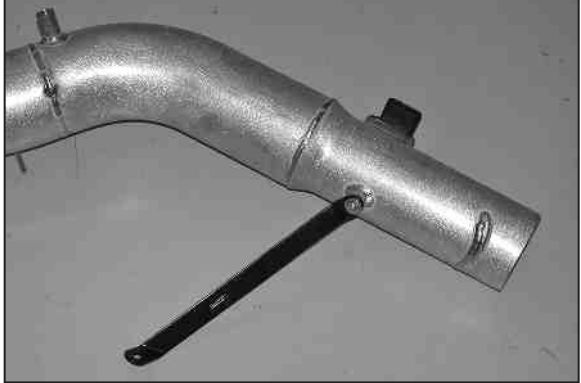
17. Install the small end of the tube-mounting bracket on the K&N® intake tube as shown. NOTE: Do not completely tighten at this time.
