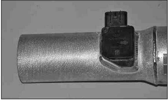
16. Install the mass air sensor into the K&N® intake tube using the factory bolts as shown.
