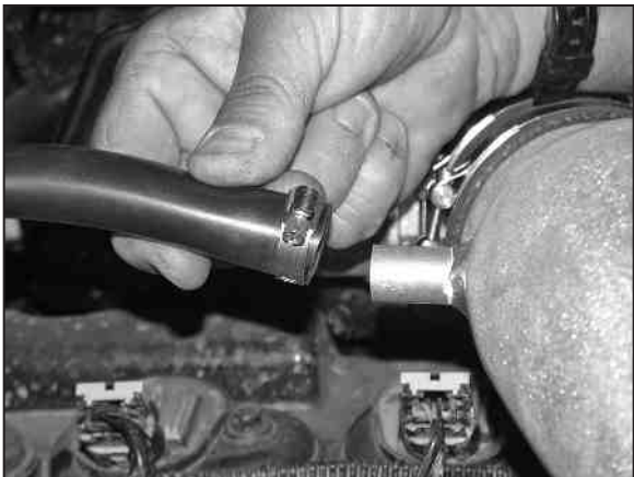
21. Install the provided crankcase vent hose onto the valve cover, then onto the K&N® intake tube as shown.
