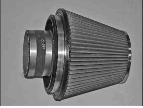
23. Install the silicone hose (08724) onto the air filter assembly as shown.
