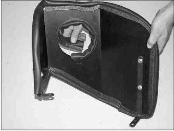
12. Install the edge trim onto the inner hole on the heat shield as shown. Trim if needed.
