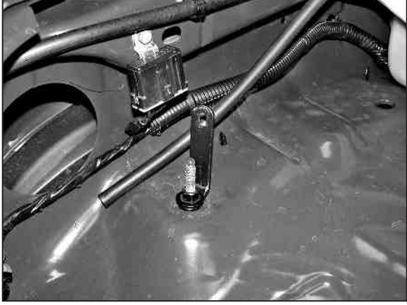
13. Install the "L" bracket (070602) onto the stock air box-mounting stud using the factory air box-retaining nut.
