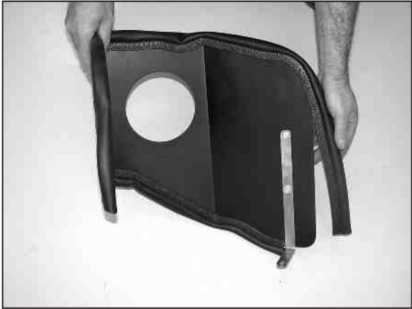
11. Install the edge trim onto the heat shield as shown. NOTE: Start the 26" edge trim at the heat shield mounting bracket on the bottom of the heat shield. Some trimming may be necessary.
