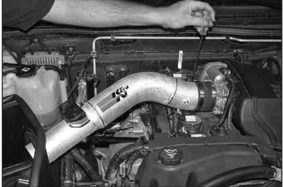
18. Install the K&N® intake tube into the silicone hose at the throttle body and through the heat shield, secure with the provided hose clamp.
