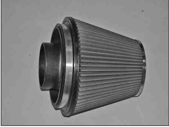
22. Install the filter adapter into the air filter and secure with the provided hose clamp.
