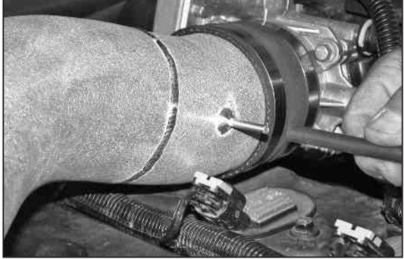
20. Install the provided 4mm vacuum hose onto the fuel pressure regulator, then onto the vent fitting on the K&N® intake tube. NOTE: On vehicles not equipped with a fuel pressure regulator, install the provided vacuum plug onto the vent fitting.
