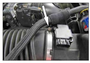
4. Loosen the hose clamp that secures the intake tube to the factory air box.
