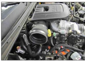
14. Install the provided hump hose (08633) onto the turbo inlet pipe and secure with the provided hose clamp.
