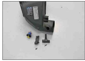
17. Remove the Filter minder and MAF sensors from the factory air box.
