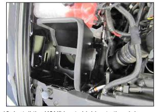
13. Install the K&N® heat shield onto the air box mounting plate and secure with the factory bolts from step #8.
