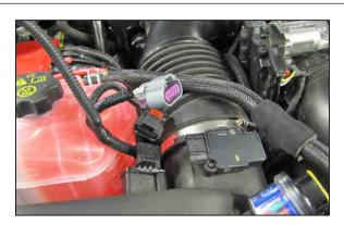
3. Disconnect the mass air sensors electrical connections and then move the harness to the side away from the intake tube.
