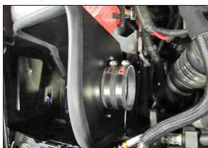
15. Install the provided hose (08761) onto filter adapter and secure with the provided hose clamp.
