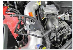
21. Reconnect the MAF sensor electrical connections and reconnect the harness connection on the intake charge tube.
