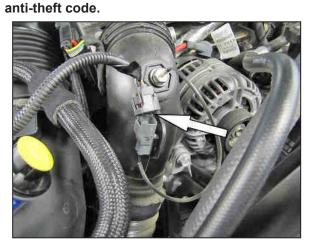
2. Disconnect the wiring harness junction connector located on the intercooler charge tube.
