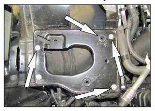
8. Remove the three bolts and the grommet shown from the air box mounting plate.
