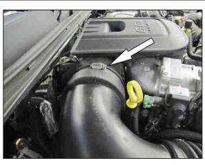
5. Loosen the hose clamp that secures the intake tube to the turbo inlet pipe.
