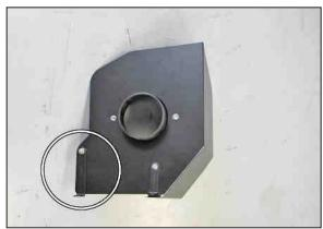
11. Install the provided "L" bracket (070952) onto the heat shield as shown using the provided hardware.
