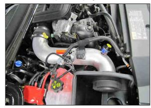
20. Install the K&N® intake tube into the hump hose at the turbo inlet and then into the hose at the filter adapter. Align the tube for best fit and then secure with the provided hardware.
