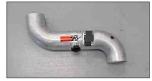
18. Install the MAF sensors into the K&N® intake tube and secure with the provided hardware. NOTE: On 2012 and earlier model year vehicles, it will be necessary to use the block off plate and gasket in place of mass air sensor.
