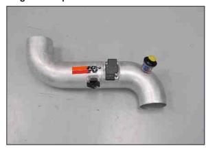
19. On vehicles that are equipped with a filter minder, install the provided grommet and the factory filter minder into the K&N® intake tube as shown. On vehicles not equipped with a filter minder, Install the provided plug.
