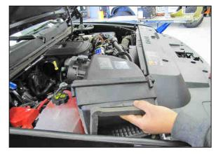
7. Lift up and remove the complete air box assembly from the vehicle.
