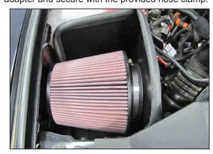
16. Install the K&N® air filter onto the filter adapter and secure with the provided hose clamp NOTE: Drycharger® air filter wrap; part # RC-5139DK is available to purchase separately. To learn more about Drycharger® filter wraps or look up color availability please visit http://www.knfilters.com®.
