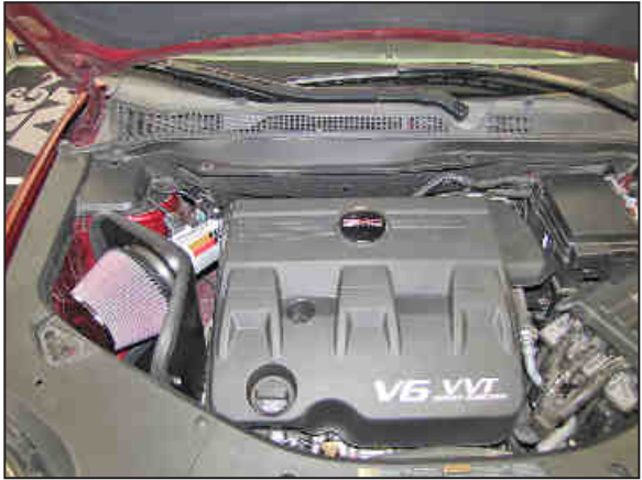
29. Reconnect the vehicle's negative battery cable. Double check to make sure everything is tight and properly positioned before starting the vehicle.
