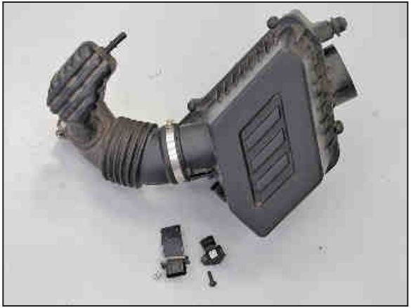
16. Remove the mass air sensor and humidity sensor from the factory air box. NOTE: Some vehicles may not be equipped with a humidity sensor.
