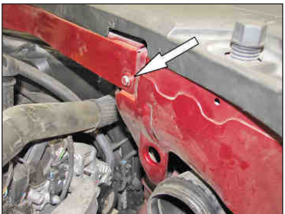
12. Remove the bolt shown in the core support.
