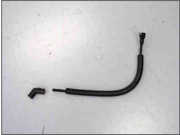
23. Remove the 45° crank case vent connector from the factory crank case vent tube.
