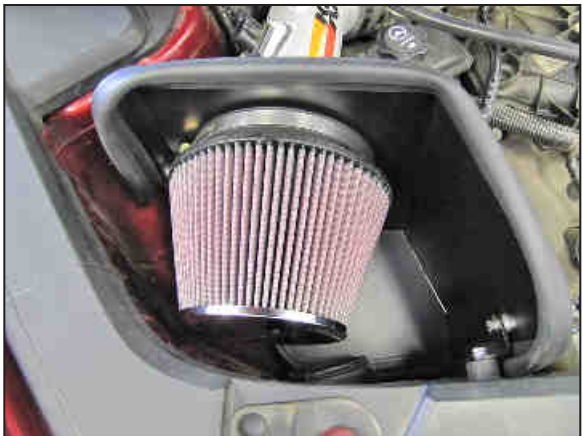
26. Install the K&N® air filter onto the filter adapter and secure with the provided hose clamp.
