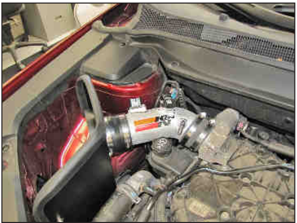
21. Install the K&N® intake tube into the hose at the filter adapter and then into the hose at the throttle body, adjust for best fit and then secure with the provided hose clamps.
