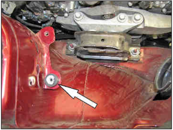
14. Install the remaining rubber mounted stud onto the air box mounting bracket as shown.
