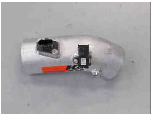
17. Install the mass air sensor and humidity sensor into the K&N® intake tube using the provided hardware. NOTE: On vehicles not equipped with a humidity sensor, install the provided block off (21568) using the o ring and hardware provided.
