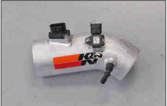
18. Install the 90° vent fitting into the K&N® intake tube as shown. NOTE: Plastic NPT fittings are easy to cross thread. Install the vent fitting “hand” tight, then turn it two complete turns with a wrench.
