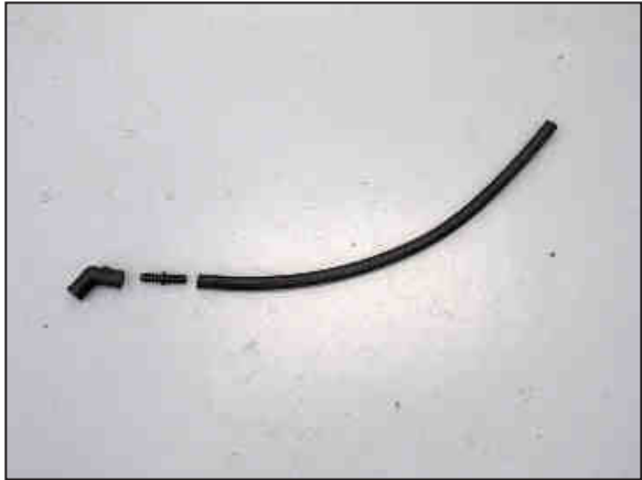
24. Using the provided hose mender, attach the factory 45° crank case vent tube coupler to the provided crank case vent hose.
