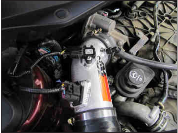
27. Reconnect the mass air sensor and humidity sensor electrical connections.
