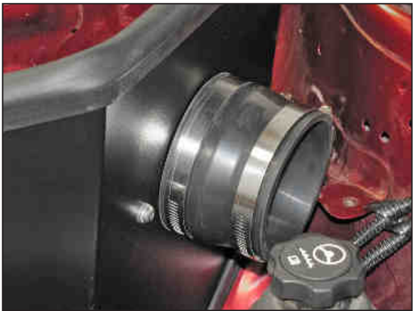
20. Install the provided coupling hose (08051) onto the filter adapter and secure with the provided hose clamp.
