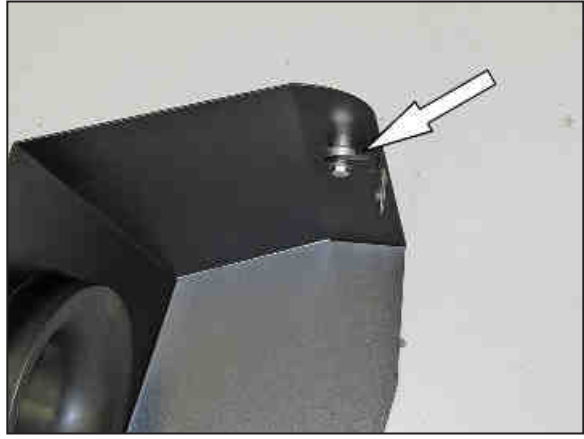
9. Install one of the provided “L” brackets (070066) onto the heat shield as shown using the provided hardware and spacer. NOTE: be sure to place the provided spacer between the bracket and heat shield.
