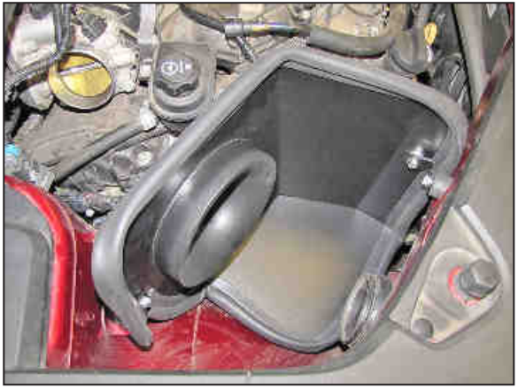
15. Set the heat shield assembly into position and secure with the provided hardware.
