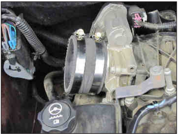
19. Install the provided coupling hose (08186) onto the throttle body and secure with the provided hose clamp.
