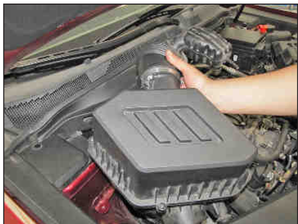
7. Lift up and remove the air box from the vehicle. NOTE: K&N Engineering, Inc., recommends that customers do not discard factory air intake.
