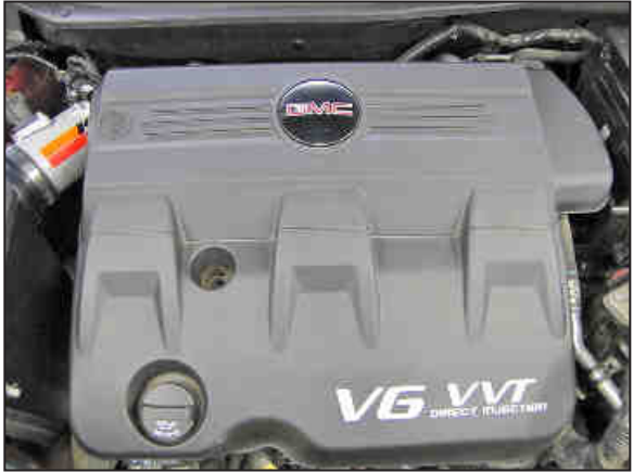
28. Reinstall the engine cover and secure with the factory bolt and oil filler cap.
