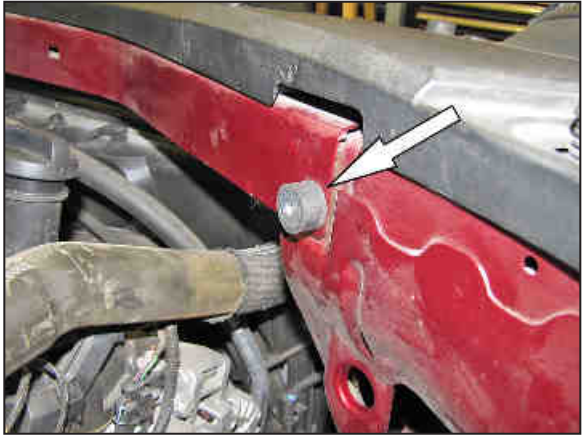
13. Install the provided rubber mounted stud into the location just vacated by the bolt removed in the previous step.
