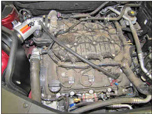
25. Install the crank case vent assembly onto the valve cover port and then onto the fitting installed into the K&N® intake tube as shown.
